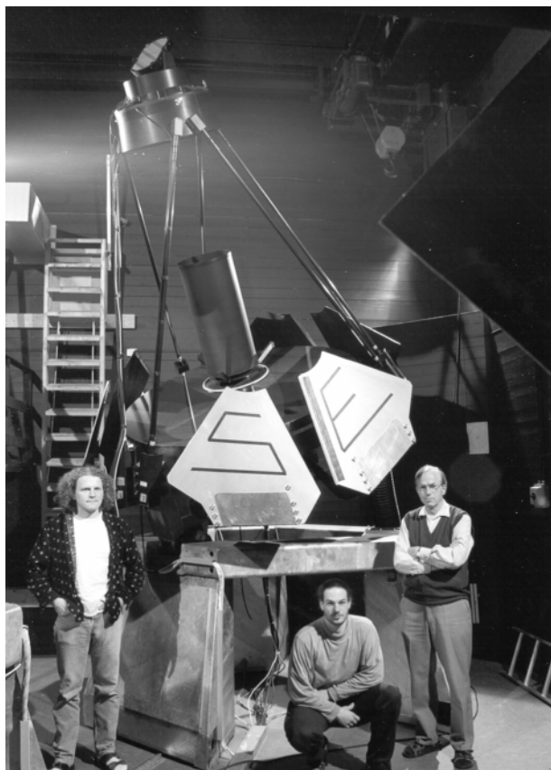
Fig. 4. The South-East telescope, in tilted position. In the centre of the figure are the 1.8 m primary and its light baffle. Six struts carry at their upper ends the secondary mirror cell and laser beam guiding mirror BGM 5. The primary is surrounded by six covers which can enclose the primary in less than 10 s. By separately moving the corners of the primary mirror cell up and down with the spindle drives, the specified tilt and azimuth angles are reached. The tiltable structure of the telescope rests on a massive hexagonal table. Persons in front of the table are (from left to right ) G. Baumgarten, D. Wagner, and U. von Zahn
