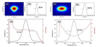
Fig. 2. (Color online) Pulse characterization at the output of the oscillator after (left) and before (right) compression. (a) Experimental SHG FROG trace, (b) retrieved pulse, (c) retrieved spectrum and spectral phase.
