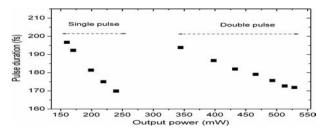
Fig. 3. Pulse duration as a function of the average output power for the 15 MHz laser cavity.
