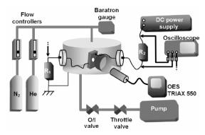
Figure 1. Experimental setup
