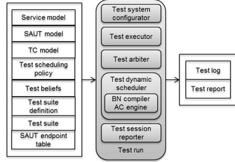
Figure 2: Automated test run with dynamic scheduling.
