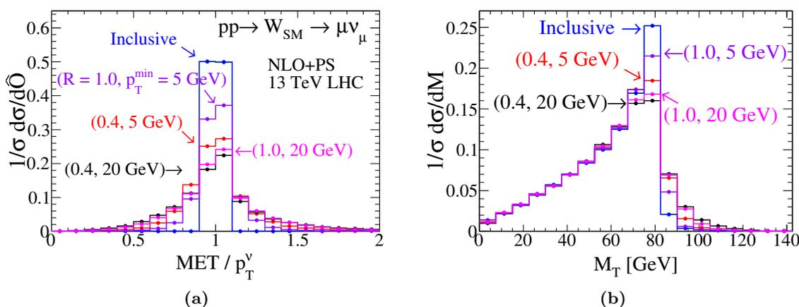
**Figure 9.** Normalized distributions for the SM process  $pp \rightarrow W \rightarrow \mu^\pm \nu_\mu$  in 13 TeV LHC collisions at the NLO+PS accuracy, with respect to (a) the ratio of reconstructed  $\cancel{E}_T$  to the neutrino  $p_T$  and (b) the transverse mass reconstructed from the  $(\ell\cancel{p})$ -system, using inclusive and exclusive  $\cancel{E}_T$  definitions and assuming various jet radii and minimum jet  $p_T$ .
