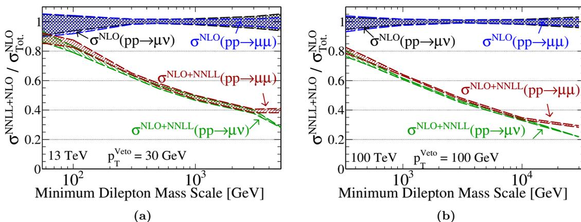
**Figure 8.** Dependence of the resummed jet-veto efficiencies on the veto scale  $p_T^{\text{Veto}}$  for the neutral current and charged current DY processes at a collider energy of 13 TeV (a) and 100 TeV (b). Basic acceptance selections on the gauge boson decay product are included, and we also show the fixed order results.
