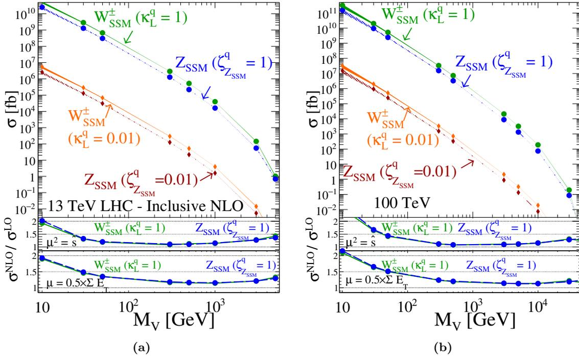
**Figure 2.** Total NLO  $pp \rightarrow W_{\text{SSM}}$  and  $pp \rightarrow Z_{\text{SSM}}$  production cross section at a center-of-mass energy of  $\sqrt{s} = 13$  TeV (a) and 100 TeV (b). The thickness of the curves corresponds to the residual scale uncertainty obtained by independently varying the central renormalization and factorization scales by a factor of two up and down.
