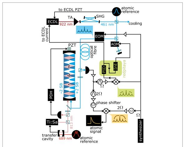
**Figure 3.** Schematic of the experimental setup. It shows the bi-chromatic high finesse cavity in which the atoms are trapped (magic wavelength at 813 nm) and probed (phase modulated laser at 461 nm). The second-order modulation sidebands form two out-of-phase standing waves in which the atoms are homogeneously coupled.
