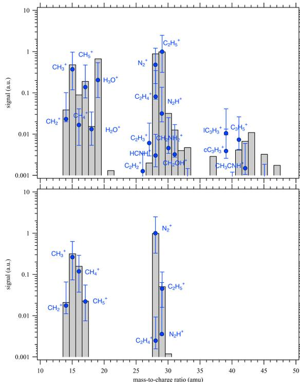
**Fig. 2.** Ion mass spectra obtained with the same experimental conditions except the pressure (*lower panel*) at 1 Pa (Bourgalais et al. 2019) and (*upper panel*) at 80 Pa in the present work. Model predictions are superimposed for each case.
