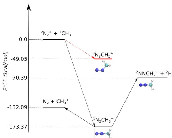
**Fig. 4.** Schematic reaction pathways relevant to the  ${}^2\text{N}_2^+ + \text{CH}_3$  reaction. In red, we report the triplet state, which is largely unlikely. The relative energies (electronic + ZPE) reported are those obtained from the CCSD(T)/aug-cc-pVQZ//CCSD(T)/cc-pVDZ calculations. For  ${}^2\text{NNCH}_2^+$ , we report the optimized structure of the most stable isomer.
