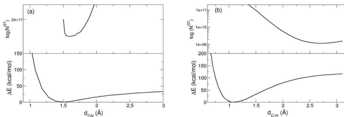
**Fig. A.2.** Internal energy and sum of rovibrational states as a function of the reaction coordinate for the two reactions studied as obtained from CCSD/cc-pVDZ energies and projected frequencies.  $N^{GT}$  values are reported for an internal energy of 174 kcal/mol.
